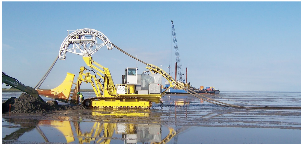
The vibration cable plough is a laying tool utilised for tidal flats © Bohlen & Doyen
